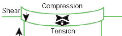
Forces applied to a beam bridge.
